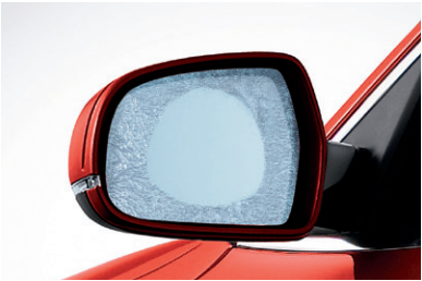
Power-adjustable, auto-dimming, heated exterior side mirrors with memory
