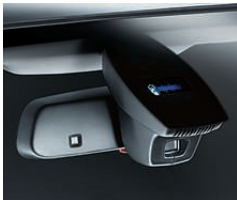
When activated, Automatic high beams switch high-beam headlights to low beams automatically when there is oncoming traffic or another car just ahead, or when the road is sufficiently illuminated. Then, when the sensor detects decreased illumination, the low beams are automatically switched back to high beams.
