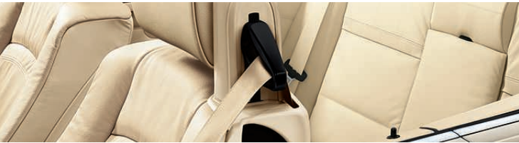
Seat-integrated safety belts help keep front-seat occupants firmly and comfortably in place. The seat-integrated design also helps ease entry and exit for rear-seat passengers.
