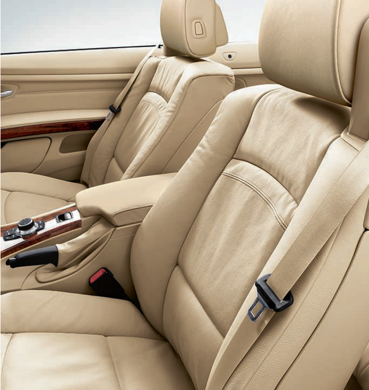
10-way power-adjustable front seats in the BMW 328i and 335i include two-way manual headrests, and can be adjusted for fore and aft position, seat height, seat angle and backrest angle. Includes two presets for driver's seat and exterior mirror positions.
