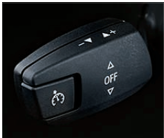
Dynamic Cruise Control 1 lets you store and maintain a chosen speed above 20 mph. It is activated via the left-hand steering column switch, and deactivated by applying the brakes or via the switch.
