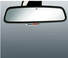
Automatic-dimming interior and exterior mirrors respond to the brightness of following headlights to minimize glare. A digital compass is integrated into the interior mirror. Both exterior mirrors are power-adjustable, with a fold-in function; the passenger-side mirror folds down to reveal the curb when in reverse gear.
