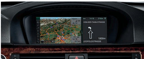
Navigation system features a high-resolution, glare-free monitor. Using GPS satellites in conjunction with data stored on an internal hard drive, a choice of detailed maps show – and tell – the directions to your desired destination. Features include 3-D daytime and nighttime maps, zoom, travel planner and an Assistance Window. In many areas, it provides Real Time Traffic Information on potential traffic problems along your route, and can even plan a detour around them. The Voice command feature can be used to change radio stations, audio selection, Navigation system destinations, and (accessory) telephone entries.
