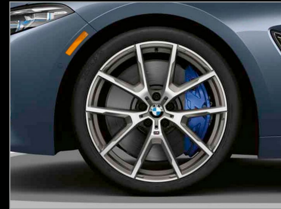
20" M V-spoke cerium grey wheels, style 728M, 20 x 8.0 front, 20 x 9.0 rear; and 245/35 front, 275/30 rear non-run-flat high-performance tires 2,3
